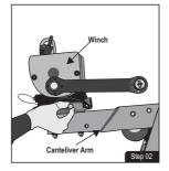
Use solid pin for locking the winch on pre-installed mounting bracket of Extreme Stainless Davit Arm.
