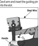
Pull out the handle of the winch outside and rotate it anti-clock wise to release the steel wire. Keep on releasing till you are able to release enough length such that it can pass over the pulleys of the Extreme Stainless Davit and get suspended vertically downwards.
